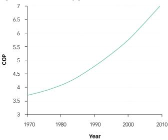
Figure 2: Chiller efficiency gains (source GHD)
